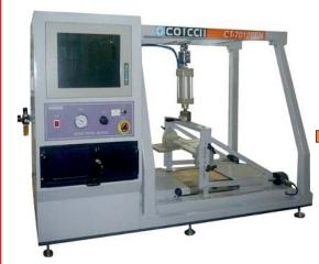
■ This machine is designed for measuring the coefficient of friction of outsole, sole forepart or heel to determine the slip resistance of a shoe. The specimen is placed on a test platform, using the glycerin as lubricant, subjected to a specified load, and then the test platform is moved horizontally relative to the specimen. The dynamic coefficient of friction is calculated after the dynamic frictional force is measured.
